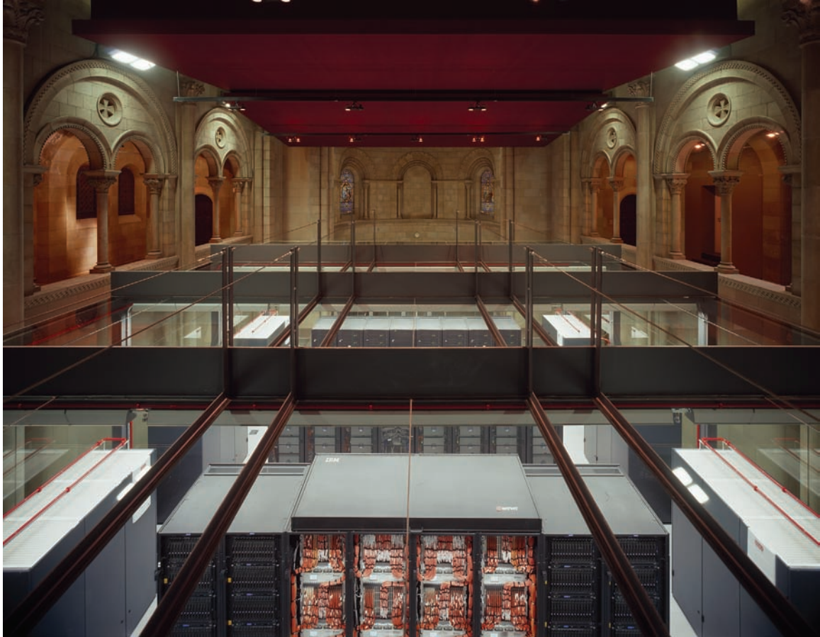
FIGURE 4-3 The MareNostrum supercomputer performs 94 trillion operations per second and includes more than 10,000 processors.
